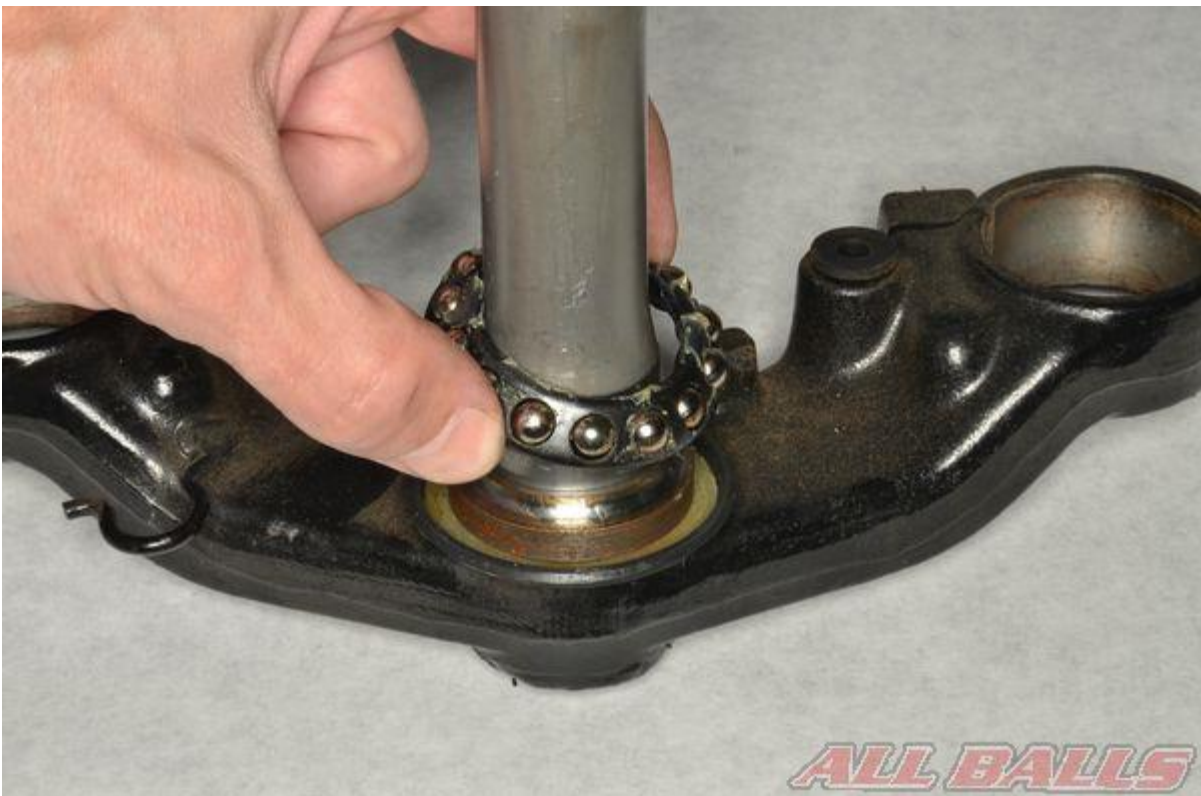
Lift the lower bearing off of the steering stem.
