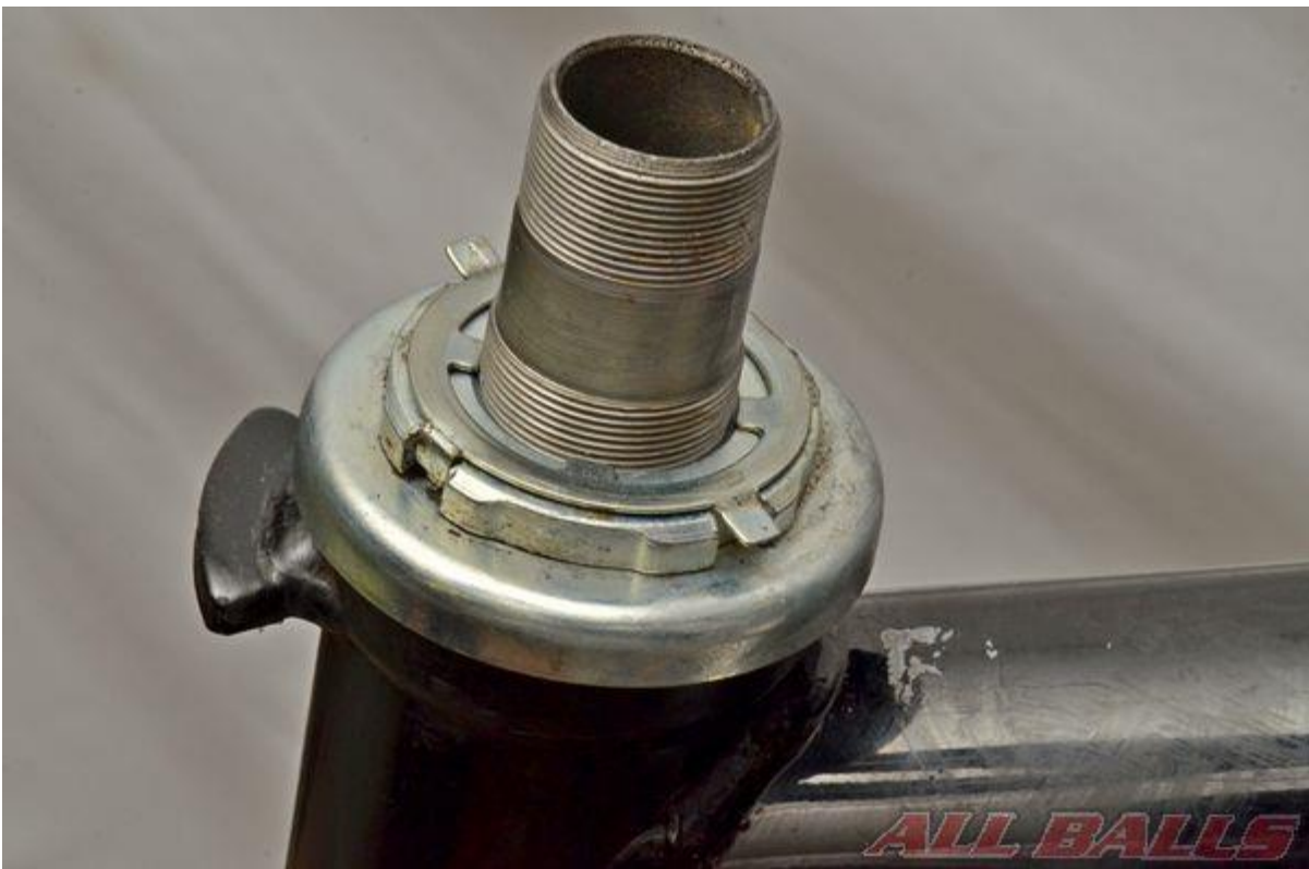
Install the new lock washer.
